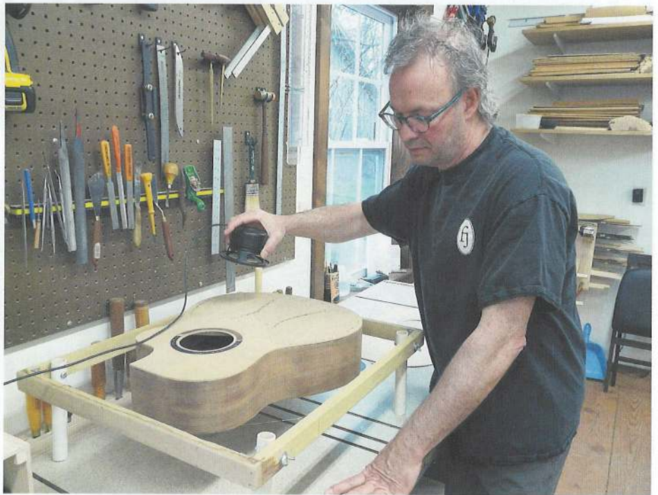
Muth places celery seeds on a soundboard and uses a frequency generator to find the vibration modes by examining the patterns they form.
