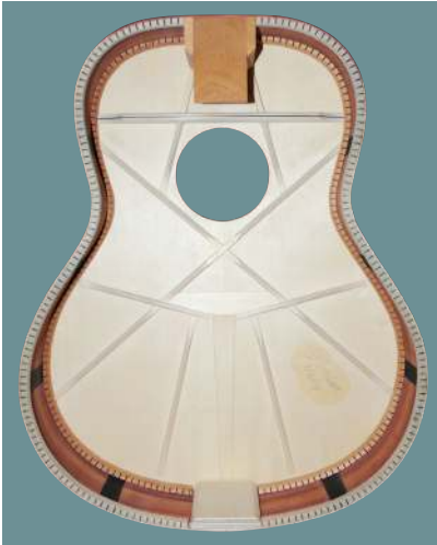
The Ascent model's hybrid X- and fan-bracing pattern.
